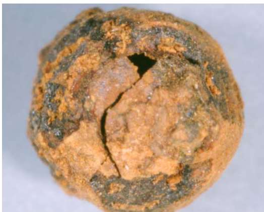
Figure 3: Spherule with hole and crack.
